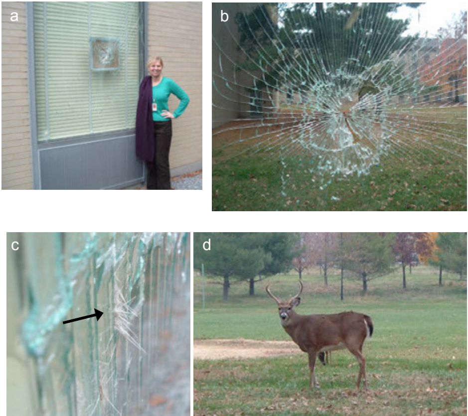
Figure 4.14 Dr. J. Quinn with a window fracture problem at NIST. Evidence collected at the scene included foreign material attached to the impact site as shown in (c). The crack patterns indicated impact from the exterior. That, plus the height of the impact above the ground, the tuft of fur, the time of the year (November, the rutting season) and similar occurrences elsewhere suggested the cause of failure shown in (d). The deer saw its reflection in the window and attacked it!
