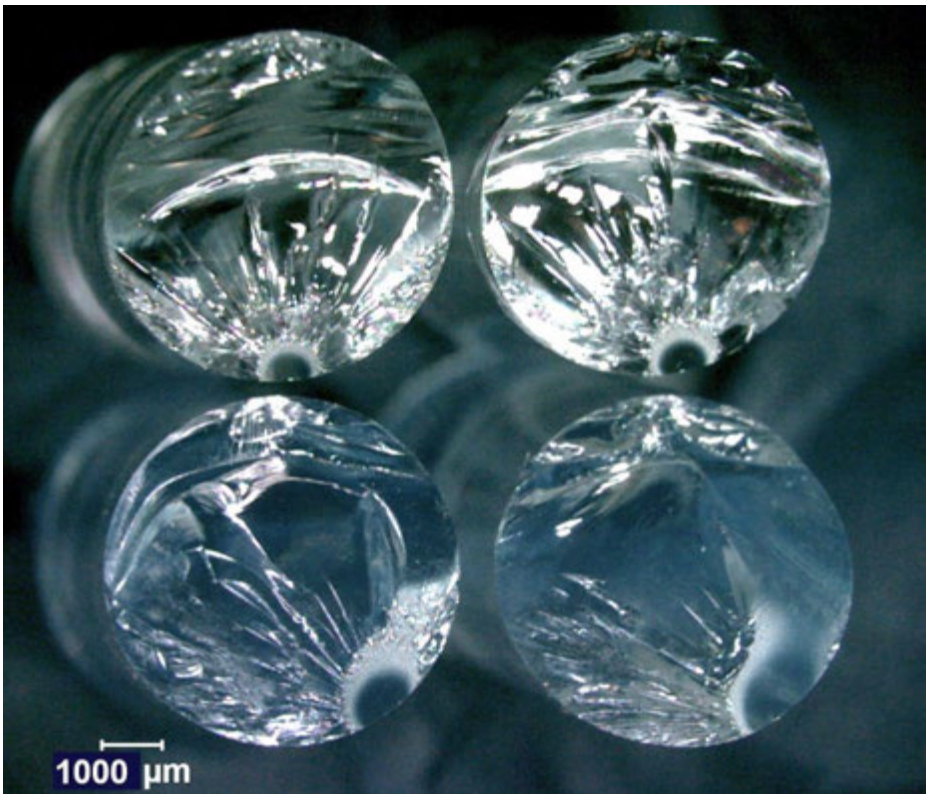
Figure 5.14 Fracture mirrors in four glass rods broken in flexure. The maximum tensile stress was on the bottom in each case. Fracture mirrors on the rod sides had pronounced flair or were incomplete due to the stress gradient.
