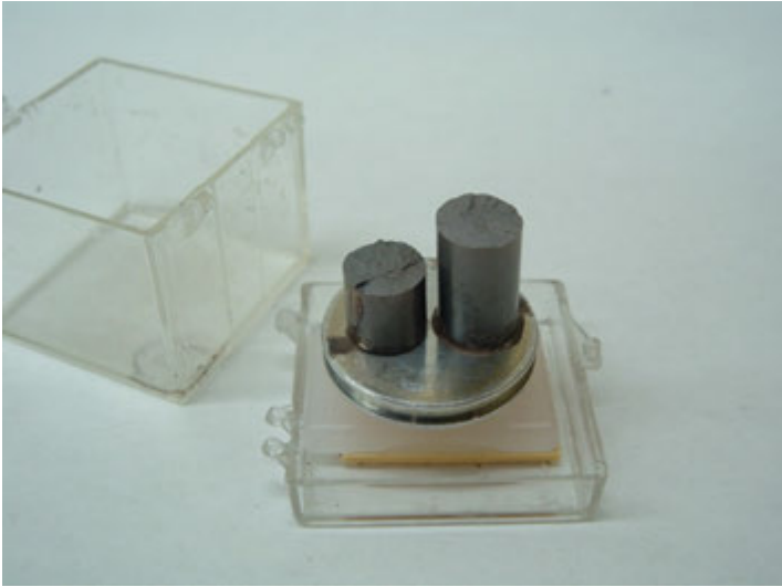
Figure 3.38 Two matching fracture halves of a broken round tension specimen on a stub in a protective plastic box. Silver paint was used to attach the specimens to the stub. Ideally, the halves should have been cut to similar lengths to save time refocusing in the SEM.
