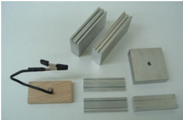
Figure 3.5 Specimen holders. Clockwise from the lower left are: a bend bar holder made with an alligator clip on a bendable (10 gage electrical) wire with electrical tape wrapped around the teeth to cushion the specimen, two aluminum jigs with slots and grooves for bend bars or tension strength specimens, an aluminum block with hole, and three aluminum holders comparable in size to a glass microscope slide with groves to hold bend bars both on their flats and on edge for chamfer examination.
