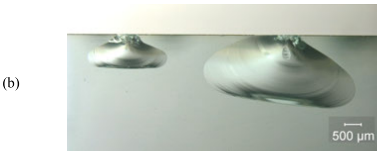
Figure 4.26 The angle of the applied load affects the shape of edge chips. (a) is a schematic that shows the patterns and (b) shows front views of two chips in glass (at different loads and distances from the edge) made by a conical indenter tool angled away from the edge at 105^\circ . (after J. Quinn and R. Mohan, Ref. 33).
