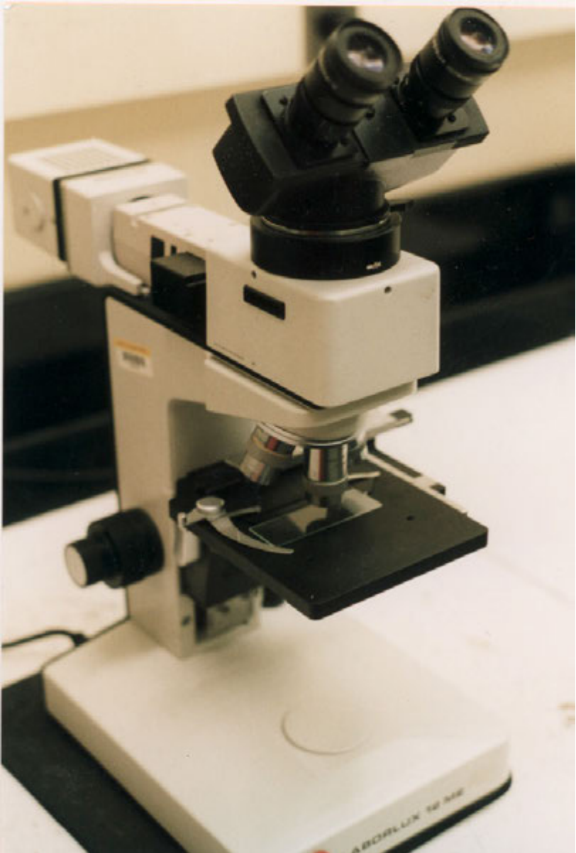
Figure 3.29 Compound reflected light microscope. Although the microscope has twin eyepieces, they both view the same image collected by the objective lens. Overall magnifications can be as much as 1000X, but the working distances and the depths of field are very small. Only relatively flat specimens may be examined.
