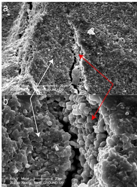
**Fig. 4 – Fractured surface of a zirconia bend bar.** The free-air sintered grains (within a fissure space) are round-shaped (red arrows) whereas the grains on a bulk fractured surface post-sintering are angulated in shape as a result of transgranular or intergranular fracture.
