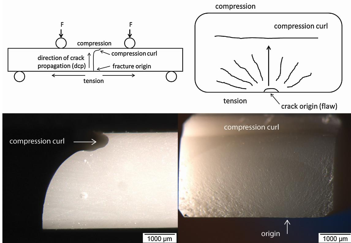
**Fig. 1 – Schematic and illustration of a zirconia bend bar under 4-point flexure test. The fracture origin is to be searched on the tensile side. A compression curl is usually easy to see and will be located at the compression side. The two stereomicroscope images show a side view (left) and fracture surface (right) of the broken zirconia bend bar.**
