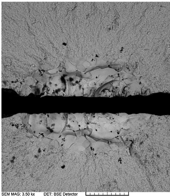
**Fig. 8 – Backscatter viewing mode of a critical flaw made of excessive grain growth in a 3Y-TZP after post-sintering HIP and 4-point bending strength test.**
