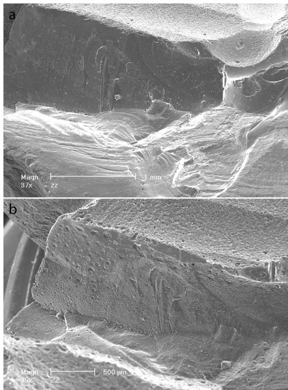
**Fig. 22 – SEM images of a clinical fracture surface of a zirconia veneered bridge with delamination of a portion of the veneering ceramic (a) as well as of a polyether replica poured with epoxy (b) both viewed in the same area. The polyether shows a poor surface reproduction of details due to its chemical incompatibility with the epoxy.**
