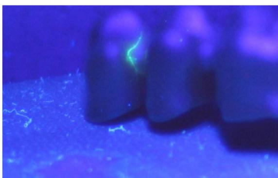
**Fig. 13 – Zirconia green body framework dipped in Ardrox® 920A, a water-washable and water-based fluorescence liquid, revealing a crack in a UV chamber (image courtesy of Diadem, F).**
