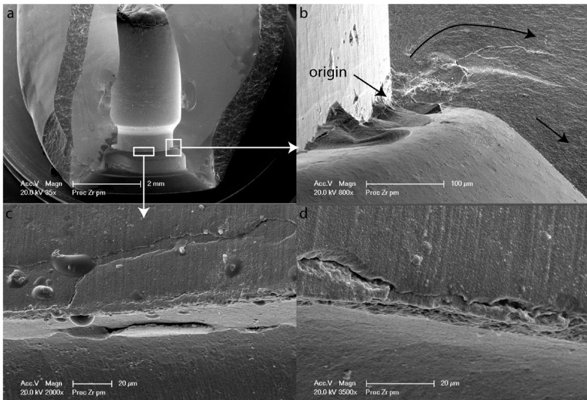
**Fig. 12 – Same case as described in Figs. 10 and 11. Further SEM analysis of the inner rim show evidence of major precracks spread over the entire length of the rim, thus weakening the structure. These cracks are related to manufacturer processing problems.**
