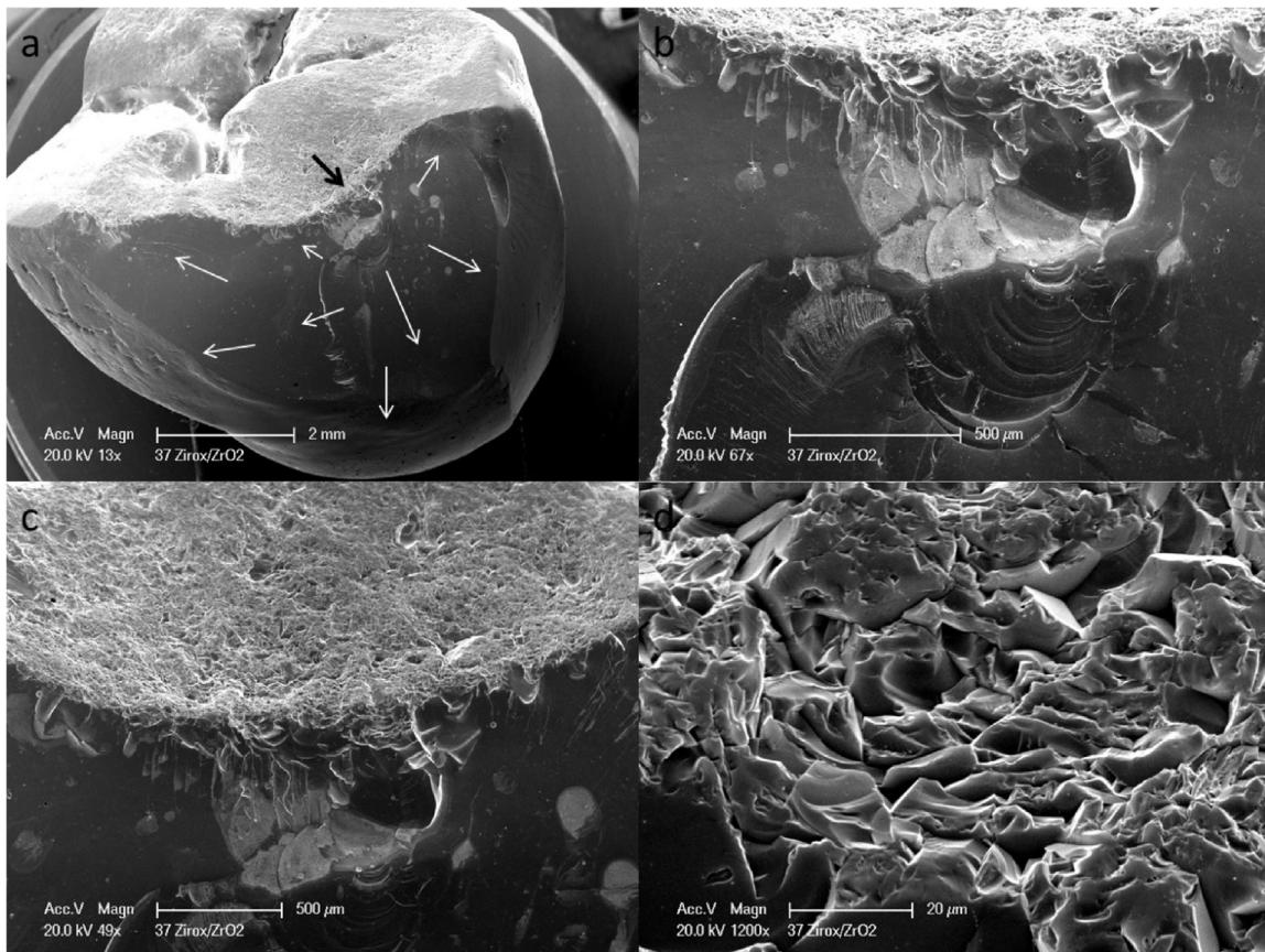
**Fig. 18 – Replica fractographic analysis of a 12 months chip-fracture of a non-leucite veneering ceramic (Zirox) over a zirconia core.** (a) Provides an overall image of both the occlusal surface and the fracture surface. The black arrow points to the origin of the chip-fracture. The white arrows indicate the dcp. Further magnifications focus on the fracture origin (b) and the substantial worn occlusal surface (brittle fracture) (c,d) involved in the fracture process.
