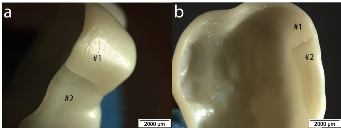
**Fig. 14 – Crack visible through transillumination on a sintered zirconia crown framework. View from the outside (a) shows a crack from the margin up along the side wall as well as through the thickness as visible from the inside (b). Note grinding marks near the margins.**
