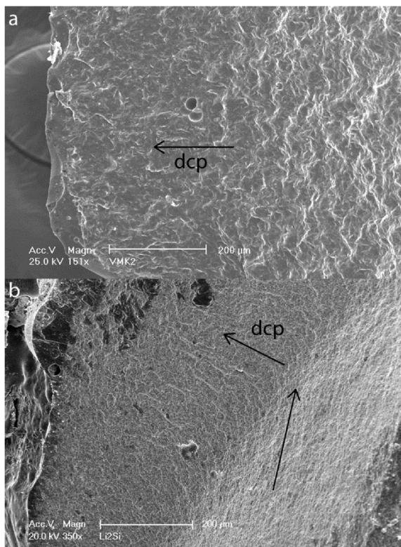
**Fig. 19 – A fractured surface of a feldspar-based ceramic (Vita Mark II) (a) and of a lithium disilicate glass-ceramic (b) is shown. Both are considered as rather difficult for identification of fractographic surface crack features and determination of the direction of crack propagation (dcp).**
