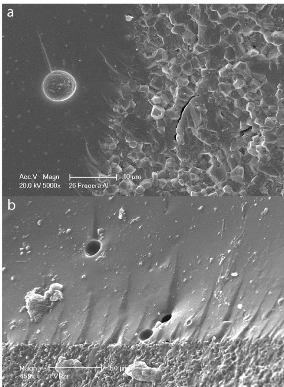
**Fig. 21 – Alumina core (a) and zirconia core (b) with their respective veneering ceramics.** The veneering ceramic in both cases show easy recognizable features such as wake hackle, hackle and twist hackle visible at the interface as a continuation of the crack front moving from the core materials towards the veneering ceramic.
