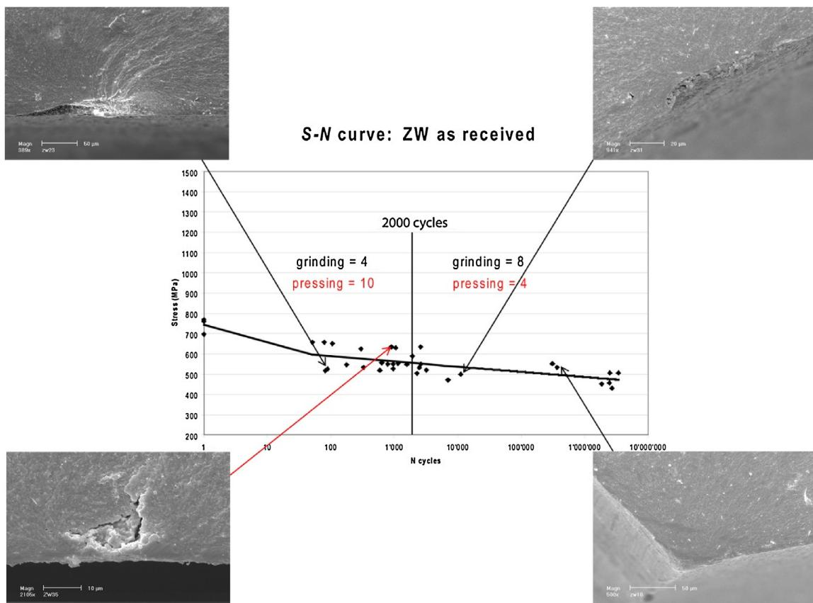
**Fig. 6 – Example of fractographically labelled S-N data.** Failure origins of selected specimens within the fatigue test are shown by SEM images. Location of fracture origins in bend bars are flaws from pressing, grinding or corner cracks (data from Ref. [42]). The red arrow is for a pressing defect on the S-N data points. (For interpretation of the references to color in this figure legend, the reader is referred to the web version of this article.)
