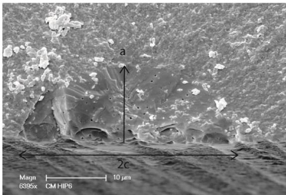
**Fig. 7 – Fracture origin in a 3Y-TZP bend bar fractured in 4-point-bending.** The critical flaw has a crack depth ( $a$ ) = 13  $\mu\text{m}$ , a crack width ( $2c$ ) = 37  $\mu\text{m}$ , a fracture stress ( $\sigma_f$ ) = 680 MPa and a calculated critical intensity shape factor  $Y_{\text{depth}} = 1.4$  using Scherrer et al. [48]. Hence, the estimated fracture toughness in this case would be  $K_{\text{Ic}} = 3.4 \text{ MPa}/\text{m}$  (data from Ref. [35]).
