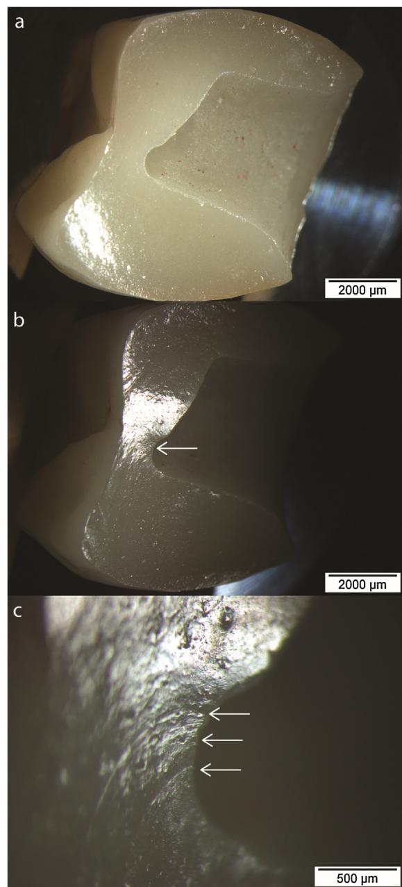
**Fig. 20 – A lithium disilicate try-in failure is documented using a stereomicroscope and lateral illumination. In (a) no fractographic features are visible in the overall image. By changing slightly the angle of light incidence it is possible to make key features to appear very clearly as seen in images (b) and (c). The white arrows indicate the crack origin failure at the inner occlusal corner.**
