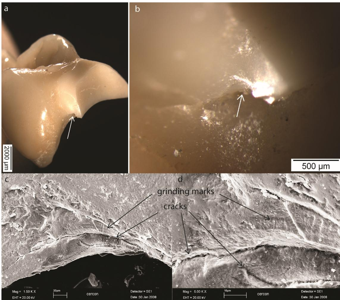
**Fig. 16 – Clinical fracture of a zirconia 4-unit bridge after 9 months of intra-oral use occurred between the premolar pontic and the molar crown abutment. The embrasure region is marked with a white arrow. Higher magnifications (c,d) show grinding marks from a bur as well as cracks. The partial fusion of these cracks indicates that cracking occurred in the presintered state.**
