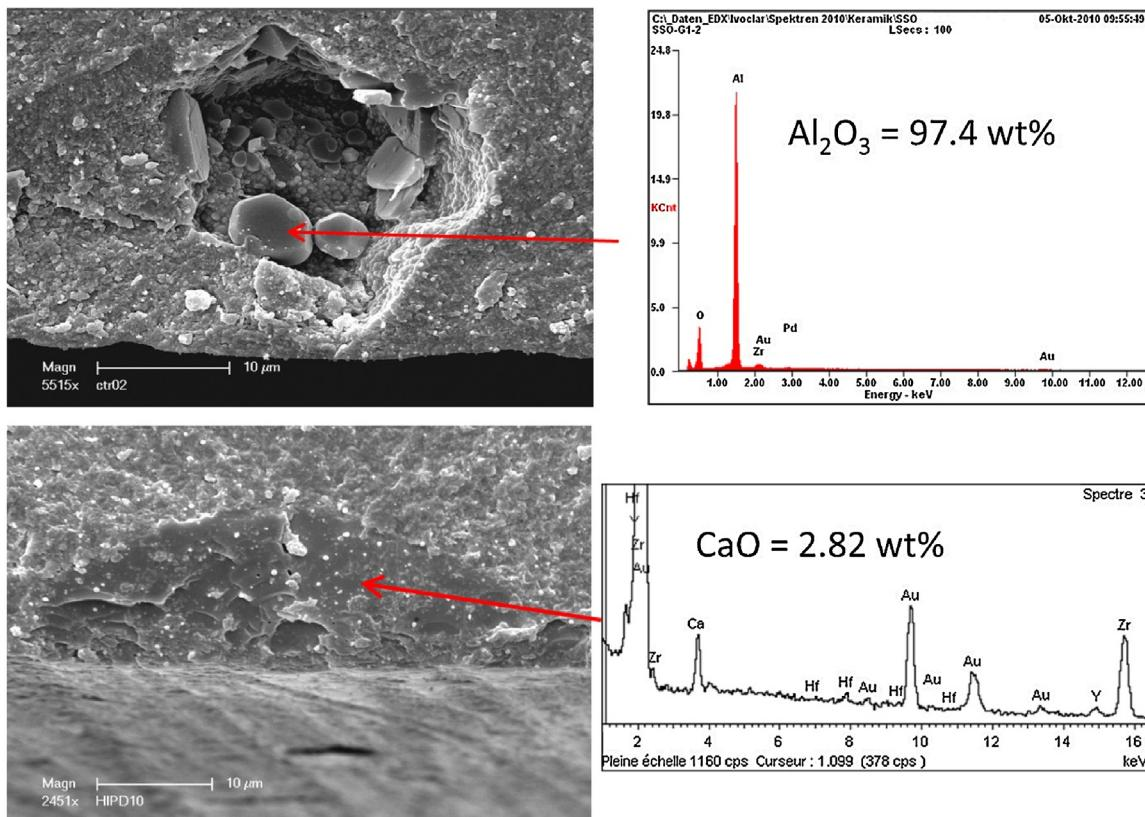
**Fig. 9 – Failure origins in 3Y-TZP bend bars. EDX combined with SEM allows identification of contaminants composition.**
