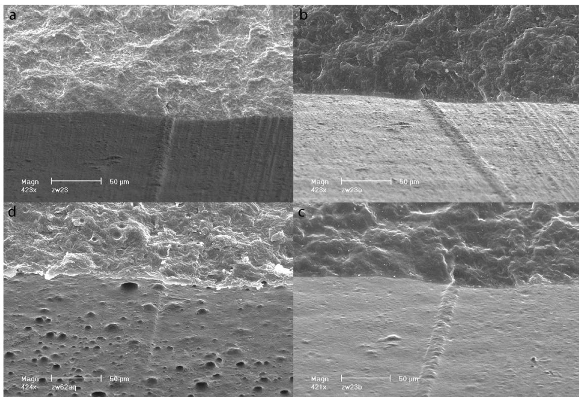
**Fig. 23 – Illustration of a detail reproduction from an original zirconia broken surface (a) and an ultralight body PVS (Express 2, 3 M) (b), a light body PVS (Express 2, 3 M) (c). Hydrogen release is shown in (d), after pouring epoxy in a light body PVS (Aquasil, Dentsply).**
